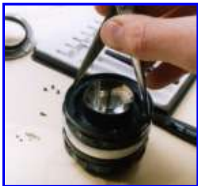
FIG. 7 - Retaining ring detachment
