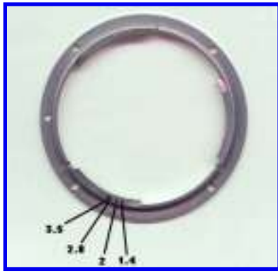
FIG. 15 - Female F-mount ring marked with some LENS SPEED INDEX POST positions.
