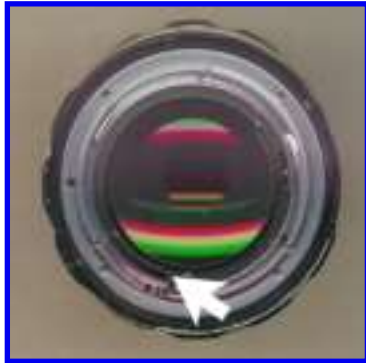
FIG. 16 - Female f-mount ring is mounted to assist LENS SPEED INDEXING POST positioning.
