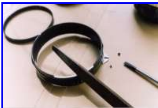
FIG. 9 - Filing the aperture ring
